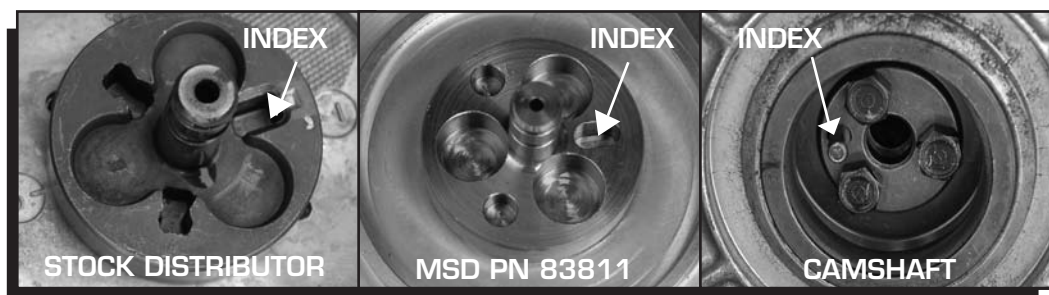
Figure 1 The Drive Mechanism of the PN 83811 Distributor.
