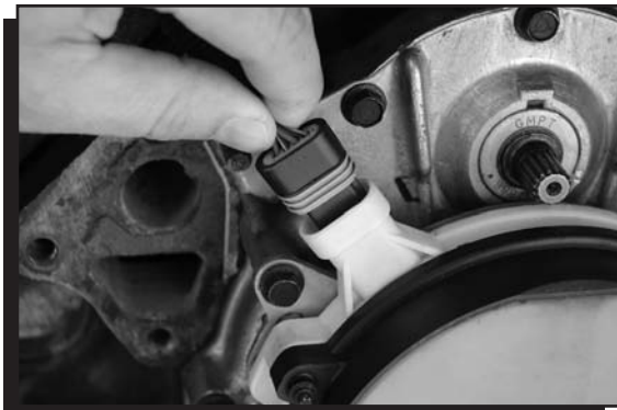
Figure 6 Disconnect the Distributor Connector.
