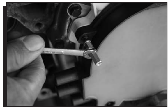
Figure 7 Removing the Original Cap.
