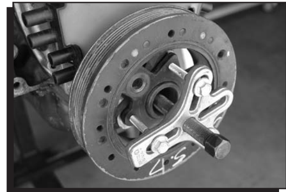
Figure 5 Removing the Hub.
