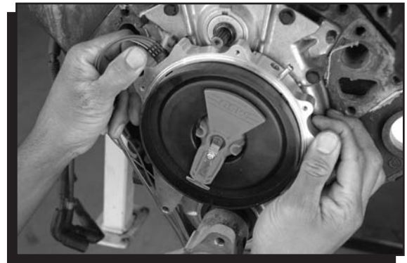
Figure 11 Installing the New Distributor.
